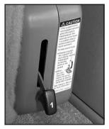
1. Pull up on the release lever labeled 1 located on the rear of the seatback, and push the seatback forward.
